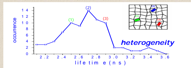
Fig 6 Distribution of single molecule radiative lifetime for 80 different Oxazine 1 molecules dispersed on \text{TiO}_2 NP coated cover coverslip
